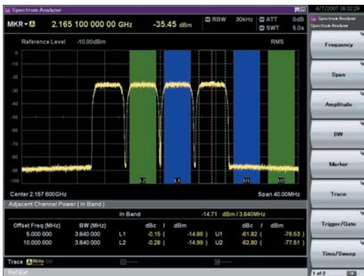
W-CDMA ACPR (Test Model 1, 64 DPCH, 4 Carrier) Waveform Pattern [Test_Model_1_64DPCH x 4]
