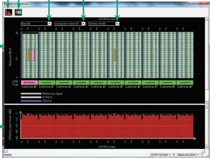
Frame Structure Screen (LTE-Advanced)
